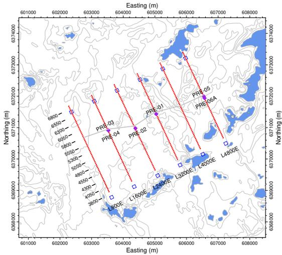
**Figure 3:** The North Grid of the 2017 MLTEM survey. The blue rectangles represent the first and the last transmitters of each profile while the red dots mark all the receivers in each profile. The purple diamond symbols represent drill holes. The gray line represents the conductor trend.
