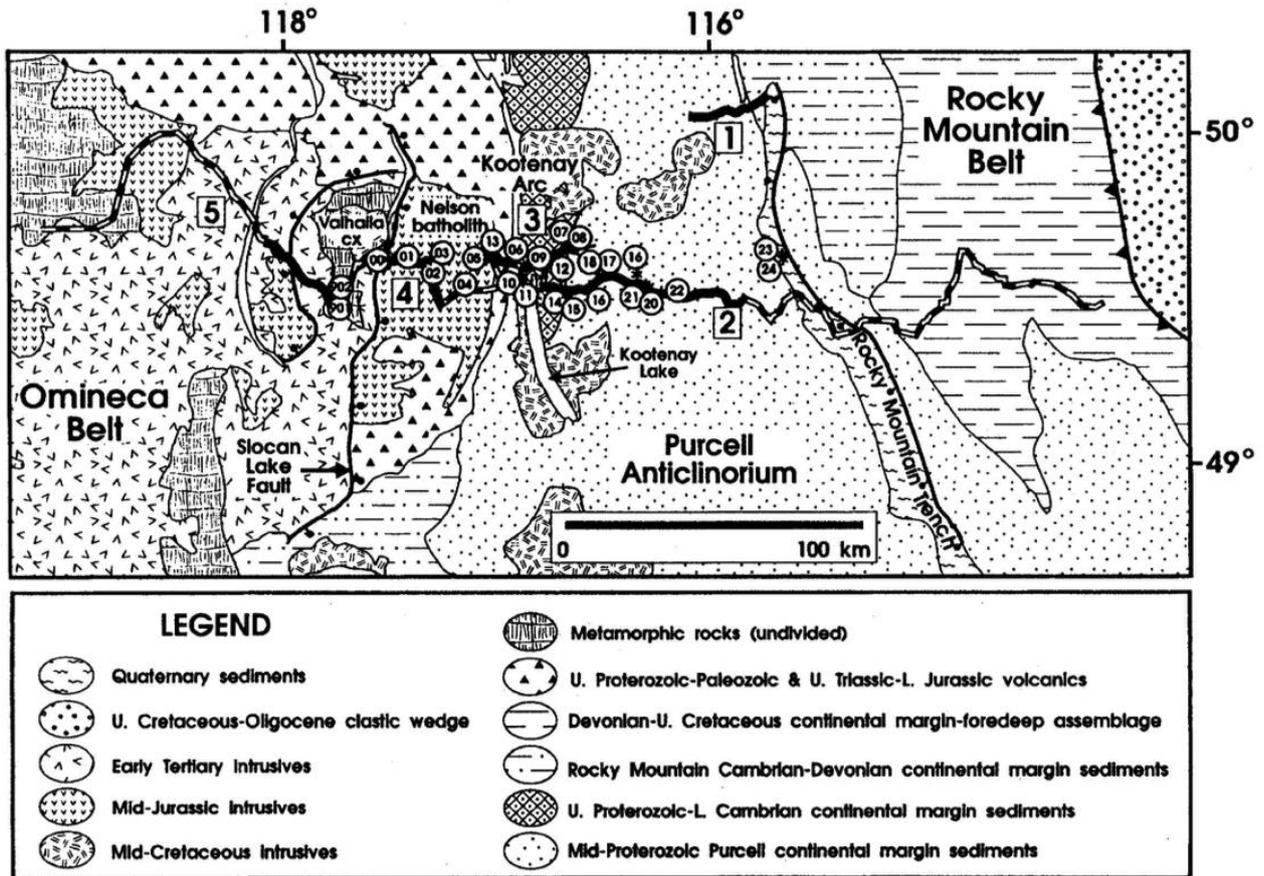
**Figure 1:** Simplified geology map of the region (based on COOK et al., 1988) showing the locations of the MT sites (numbers in circles), the seismic reflection lines (solid lines with associated numbers in squares) and seismic refraction receiver points (dashed line). Overlapping circles indicate local/remote 10-channel pairs.
