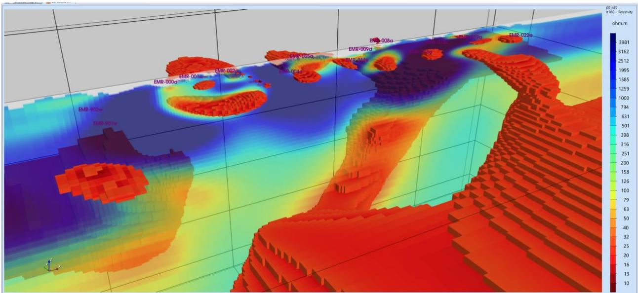
**Figure 4:** Current best 3D model to the BC87/EMAP88 data. The solid surface is 30 Ωm.
