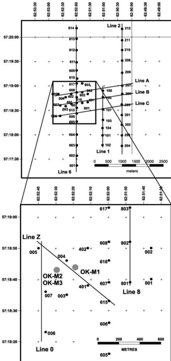
**Figure 6:** Map of AMT site locations in the Okak Bay deposit area. The AMT sites were assigned to the nine profiles shown (0, 1, 2, 6, 8, A, B, C, Z). Also shown are the locations of the drillholes OK-M1 and OK-M2/OK-M3.
