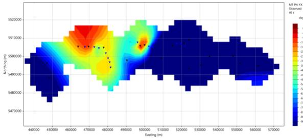
**Figure 3:** Out-of-quadrant PhaYX phases at 46 s period.
