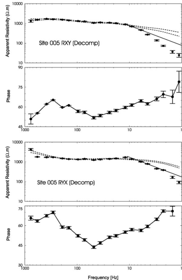
**Figure 7:** Derived low-frequency tensor decomposed apparent-resistivity data for site 005 together with their prediction (dashed lines show  $\pm$  one standard error) from the phase data using Parker and Booker’s (1996)  $\text{Rho}^+$  algorithm. The solid lines in the apparent resistivity plots show the decay for an infinitely conducting substratum. Also shown are the decomposed phase data.
