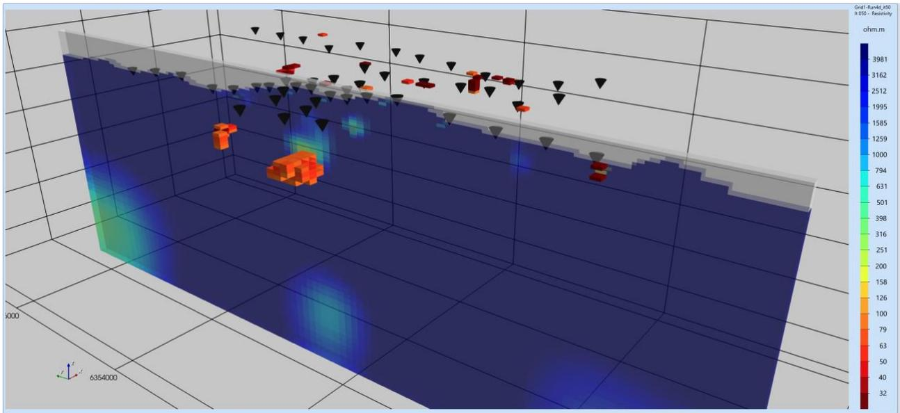
**Figure 8:** Current best 3D model of the Okak Bay dataset. The surface is at 100  $\Omega$ m, and the slice is along Line 6. View from the SW towards the NE.
