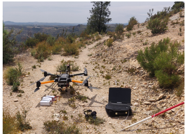
Figure 1: UAV with SHFT sensor attached in survey area north of Huelva, Spain.
